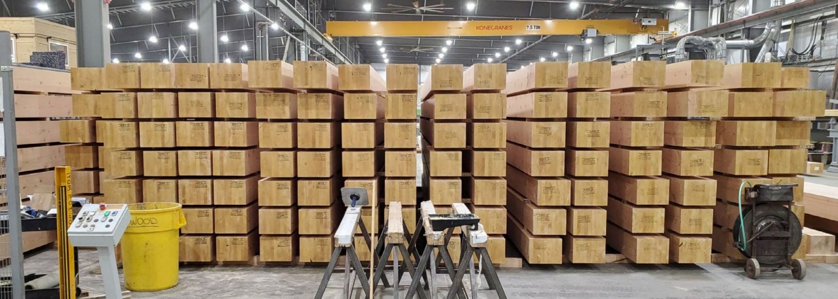
ABOVE PCC Metro Center's glulam members in the fabrication facility before delivery onsite (Photo credit: Kalesnikoff)
