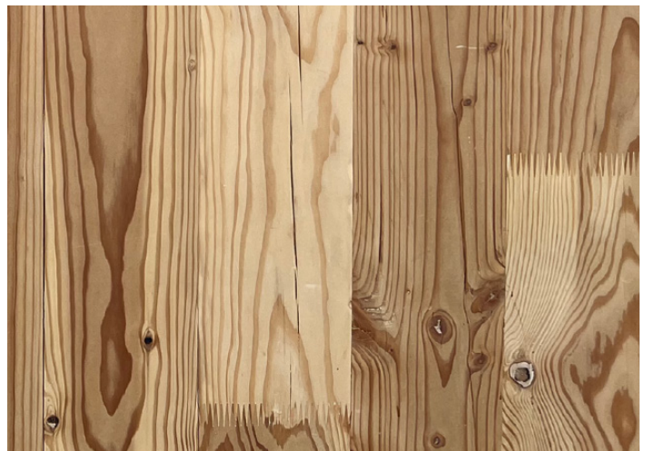
ABOVE Looking closely at the finished surface of CLT, one can see many small imperfections like checks and knots that are deemed acceptable within standard limits. Also note the "finger joints" just above and on the right.
