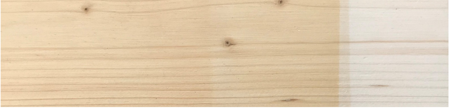
ABOVE This piece of CLT was exposed to UV light through a modern window. The left side was exposed to light for 170 days, the center for 30 days, and the right was protected from light. The degree of tanning shows that most of the effect occurs within the first month of exposure. The wood color equalized when exposed uniformly for another two months.
